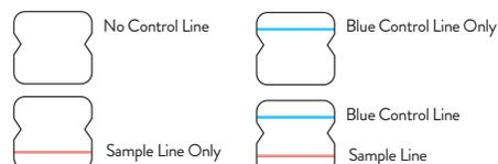
If no lines are seen, or if just the Sample Line is seen, the assay is invalid. Invalid tests should be repeated with a new swab and a new test device.
