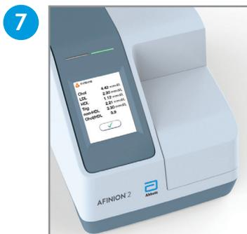
Record the result when it appears on the screen. Touch
