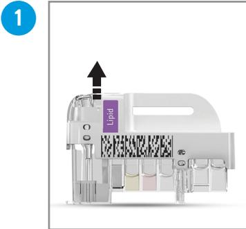
While holding the test cartridge by the handle, turn it upside-down once and return to normal position before use. Pull the sampling device straight up from the test cartridge.
