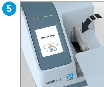
5 Insert the test cartridge with the barcode facing left.
