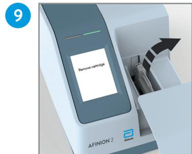
9 Remove and immediately discard the used test cartridge. Close the lid manually when the analyzer is not in use.
