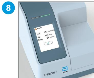
8 Record the result when it appears on the screen. Touch to accept. The lid opens automatically.
