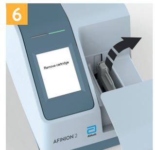
The lid opens automatically. Remove and discard the cartridge.
