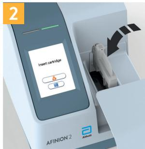
The lid opens automatically. Insert the test cartridge. The barcode should face left.
