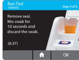
**Vigorously mix the swab in the liquid for 10 seconds.** Press the swab head against the side of the Sample Receiver as you mix it. This helps remove the sample from the swab. Once the swab is removed, touch 'OK' to proceed.
